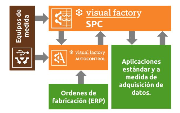
One of the main characteristics of the Visual Factory SPC system is its connectivity and integration with other systems present in the industry nowadays. Some of these systems are listed below and will be further explained:
